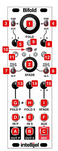
2. XFADE knob - Controls the relative mix of the two folders present at the MIX [C] output. When fully counterclockwise, only the Parallel circuitry is heard at the MIX out. Turning the XFADE knob clockwise crossfades from the Parallel folder to the Serial folder, with both circuits
