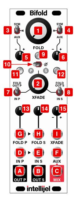
**AUX -** When set to AUX (down position), the **AUX [F]** input is added to the **IN P [D]** signal (after being attenuverted by the corresponding knob [5]). Note that if nothing is connected to the **AUX [F]** jack, then the signal appearing at the **MIX [C]** output is used as the AUX input.
