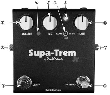
ON/OFF FOOTSWITCH: (#1 on above diagrams) When pedal is ON, the LED (#4) will be lit. The ST-Jr utilizes True-Bypass switching via the Fulltone 3PDT footswitch.
