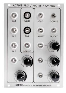
The Serge **NOISE SOURCE (NOI)** generates both white and pink noise waveforms. The S/H Source output produces the necessary input for a sample and hold function to produce equi-probable random voltages, similar to a 1/F distribution function and is a perfect companion for the Smoothed & Stepped Generator (SSG).
