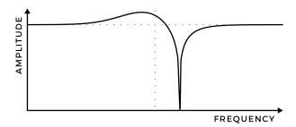
Next is the phase shifter output. It consists of a 3-pole allpass response, mixed together with the input signal. This creates a combined highpass and notch response, essentially a one-stage phaser effect. It will resonate at 315°.
