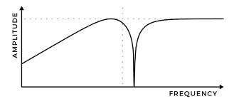
The final pole-mixing output is a 4-pole bandpass response, selecting a band of frequencies around the filter frequency. It will resonate at 360° (equal to 0°, so no phase shift).
