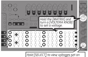
Hold (SELECT) to view voltages set on this Voltera. Press a lit (MATRIX) button to clear the step.
