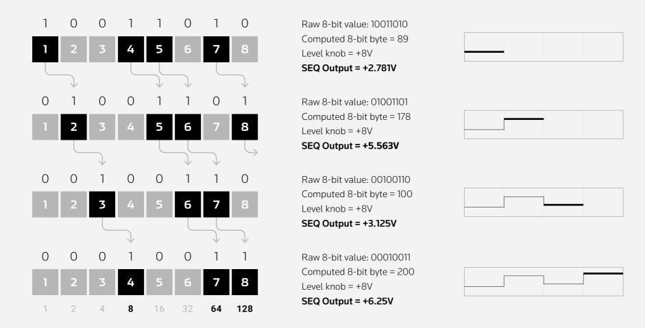
The random CV sequence is generated by evaluating the first eight bits of the shift register and calculating their value as an 8-bit "byte" (a basic concept of digital computation). Each bit has one of two states, and there are eight bits, so the output range is 2^8=256 discrete values.
