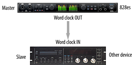
Figure 5-20: Slaving another digital audio device to your MOTU device (an 828es in this example) via word clock. For the 828es clock source, choose any source besides word clock, as it is not advisable to chain word clock.
