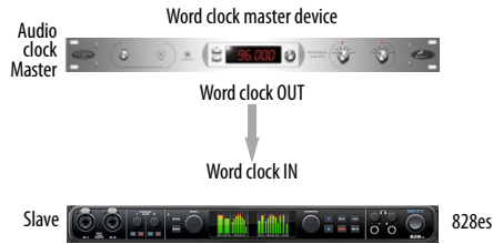
Figure 5-21: Slaving your MOTU device (an 828es in this example) to word clock. For the 828es clock source, choose 'Word Clock In'.
