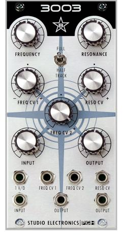
$^{\star}$  From 7:00 (0) to 9:00 our "Negative Resonance Saturation" adds beefiness, boosting the waveform amplitude and taming waveform transients; set to 9:00 to achieve the cleanest tone possible.
