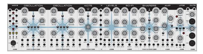
Modstar Seito Rising 106 hp: MIDI 3 6hp, Router (R—not pictured) 2hp, Oscillation (x2) 32hp, 4075 12hp, M 2hp, Levels 10hp, Sci-Fi 10hp, Shapers 12hp, Amp 8hp, LFO 2 6hp, Outs 6hp. Housed and powered in a sleek and sturdy, carbon-fibre black MONOROCKET M6E case.
