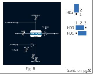
Please Note: When the VCA is configured to filter output it will block the sound, only by applying a CV to the VC-Gain input will it open the VCA for sound to pass through.
