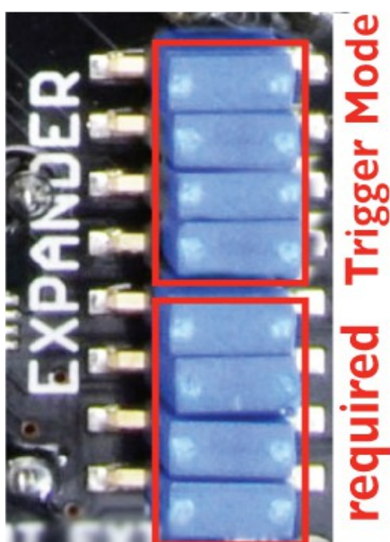
Trigger Mode: Install all eight jumpers
