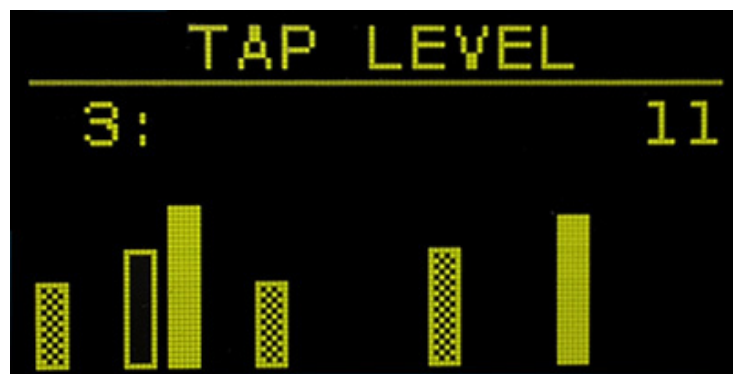
Figure 6. An example of the display when editing the LEVEL parameter for tap #3. Taps 1, 6, and 10 are muted. The tap number (3) being edited is shown in the left hand part of the second line of text, and the value of that tap's LEVEL parameter (11) is shown in the right hand part of the second line of text.
