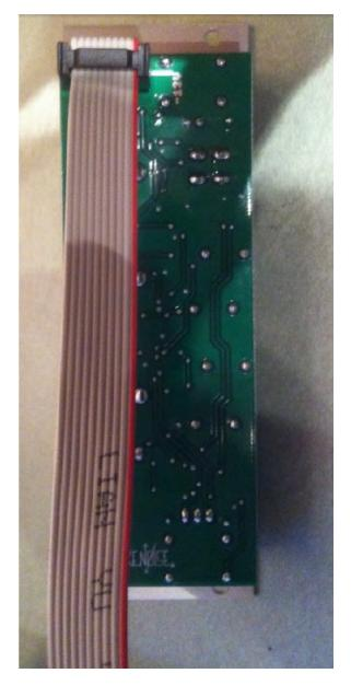
Proper installation of included power cable on module. Please note the RED BAND.
