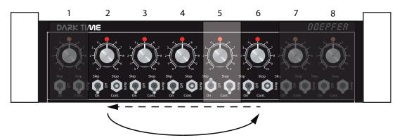
The sequence is running from step 2 to step 6 (first and last steps on "Jump"-position). Step 5 will not generate a trigger-signal ("Skip"). Step 4 (also on "Jump"-position) does not affect the sequence.
