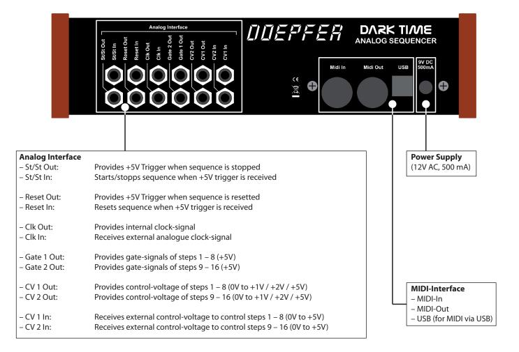
The following picture shows some kind of "**basic setting**". When the panel functions are set to this, Dark Time will play two parallel 8-note sequences with all steps at equal pitch and length. Control voltages of 1V/octave scaling (the common standard) are putted out, the step-knobs are quantised which means their range is divided into descrete half-tone steps. Dark Times tempo is internally controlled resp. controlled by the clock-knob. Step length is equal for all steps.
